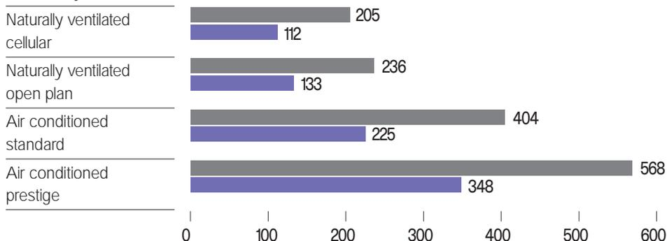
Figure 10 Carbon dioxide emissions benchmarks for office buildings (Source: CIBSE Guide F)
